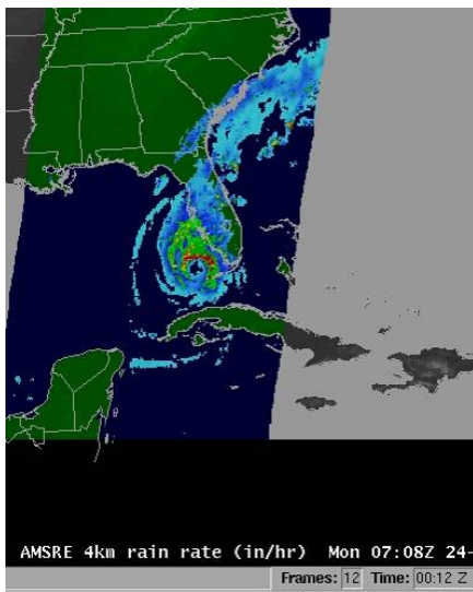
An AMSR-E rain rate product displayed in AWIPS D2D software package indicating rain intensity of an off-shore tropical system.
